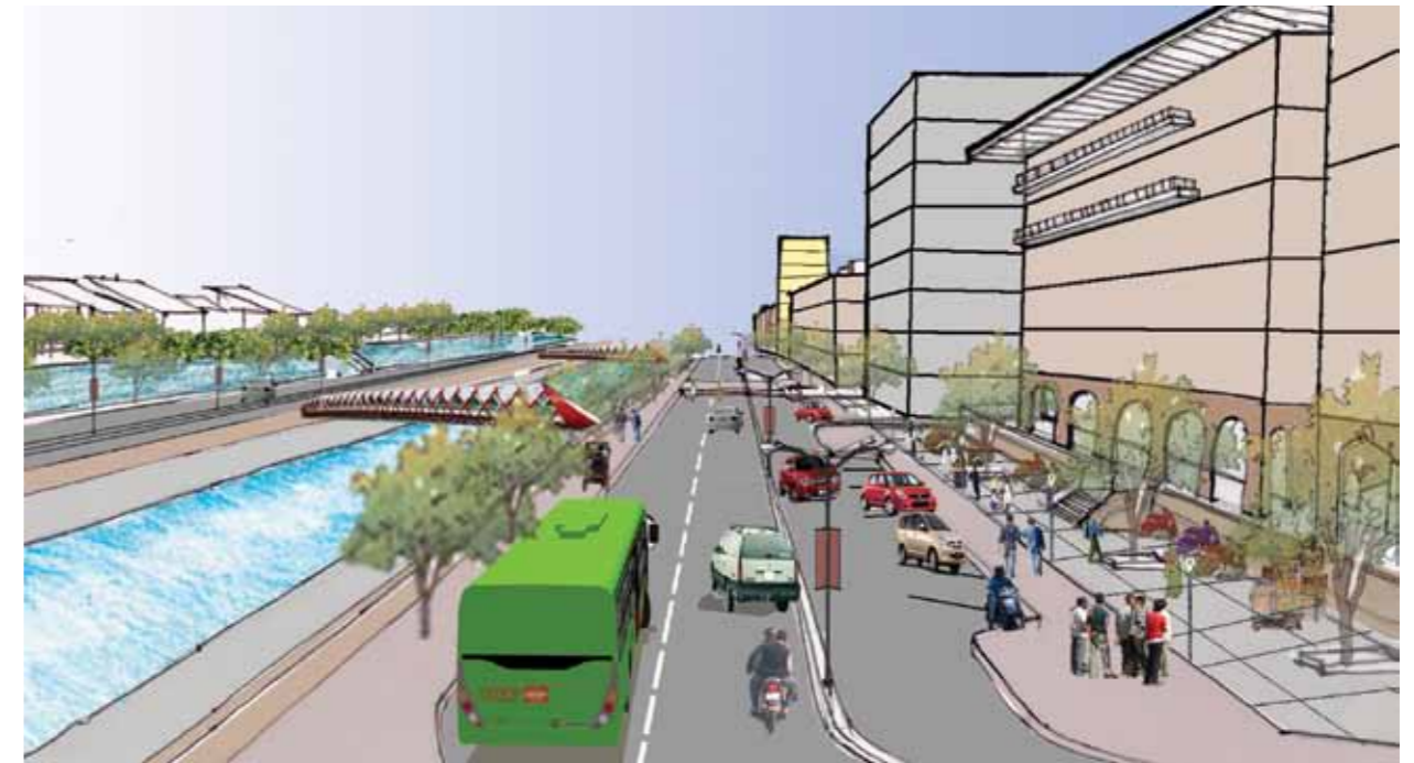
Proposed Canal Road with redeveloped built edge, reorganized street space with parking, NMV and pedestrian areas, bus lanes
